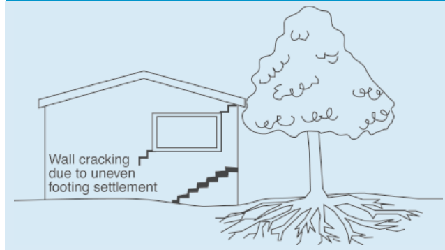
Trees can cause shrinkage and damage
